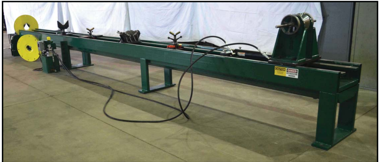
HCRS 1C CYLINDER REPAIR BENCH
