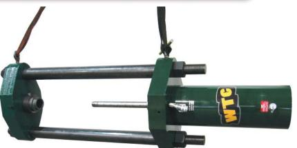
The MPP250 press is available without a hydraulic pump, or we provide several durable pumps to match shop or a service truck power. For safety during use, we also offer an optional pressure gauge, lifting sling (engineered specifically for use with this press) and a safety blanket (to protect from possible flying debris).
