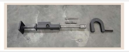
HFPP consists of: Hands free punch for pin diameters 1.4 (36mm)" and larger Medium Tool Holder for pins 1.1 (28mm)" to 1.4 (36mm)" Small Tool holder for pins 0.7 (18mm)" to 1.1 (28mm)" Heavy U-Clamp
