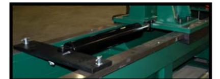
62-029A CYLINDER ASSIST ASSEMBLY, NO TUBE
